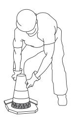
Figure 35-E. Slump Test (Cone Invert)
